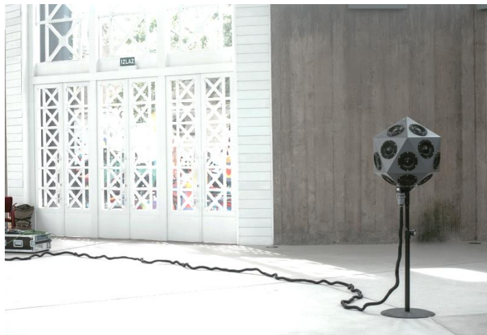
Figure 1: The IKO with stand and amplifier
